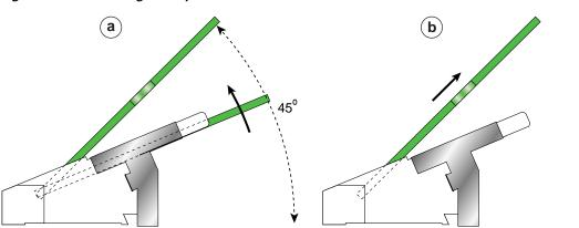
Figure 53 Removing a 144-pin SODIMM Module
